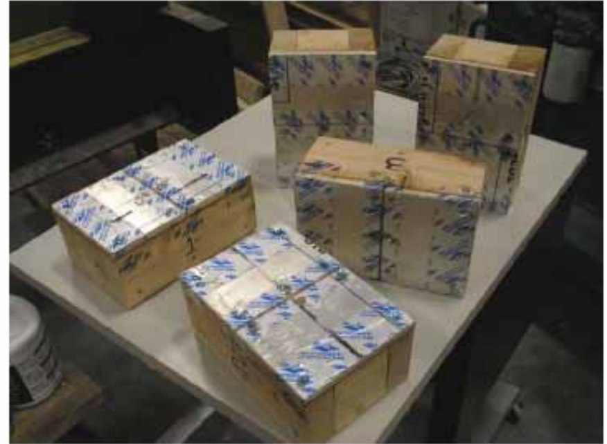
PHOTO 4: Small specimens after freeze-thaw testing in accordance with AC212 Section 4.2.
