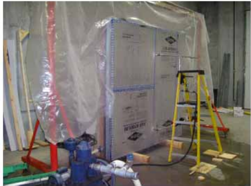
PHOTO 12: Specimen with spray rack for water penetration testing in accordance with ASTM E 331.
